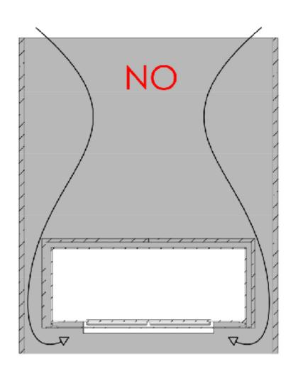
DO NOT! install the fireplace in a wall construction which is open above and below the fireplace. The warm air will cause turbulences inside this hollow construction which will have a negative impact on the flames.
